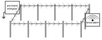
\*The Fence-Alarm senses voltage from both sides of a loop-back fence, so it will not send an alert of a broken fence line. It will however notify you if voltage drops below your threshold settings, or if your energizer ceases to function.
